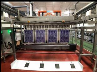
The system starts with an "Insoluble Anode System" for enhanced operational acid copper plating. It runs off of a Copper Oxide Feeder System that allows for consistent plating since the copper is continually replenished. The consistency is measured by the Inline Colorimeter.
