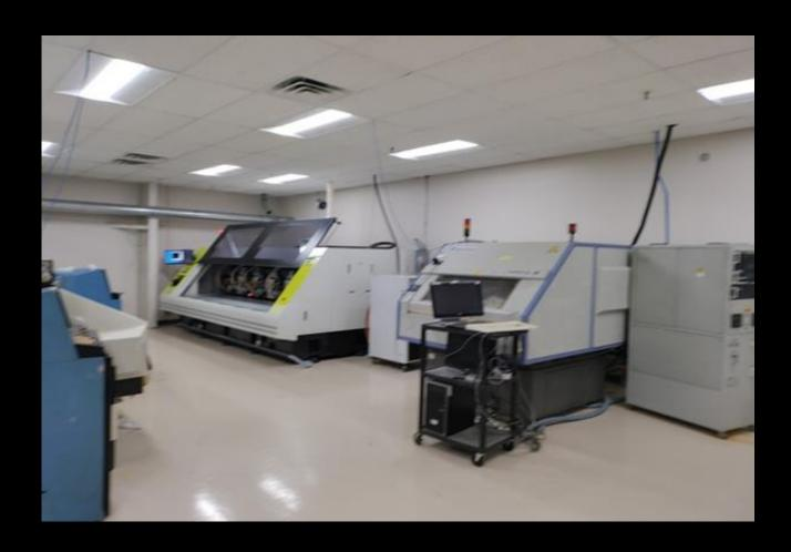
X-ray targeting measures all inner layer four corner targets and averages the distance for optimal hole location.
